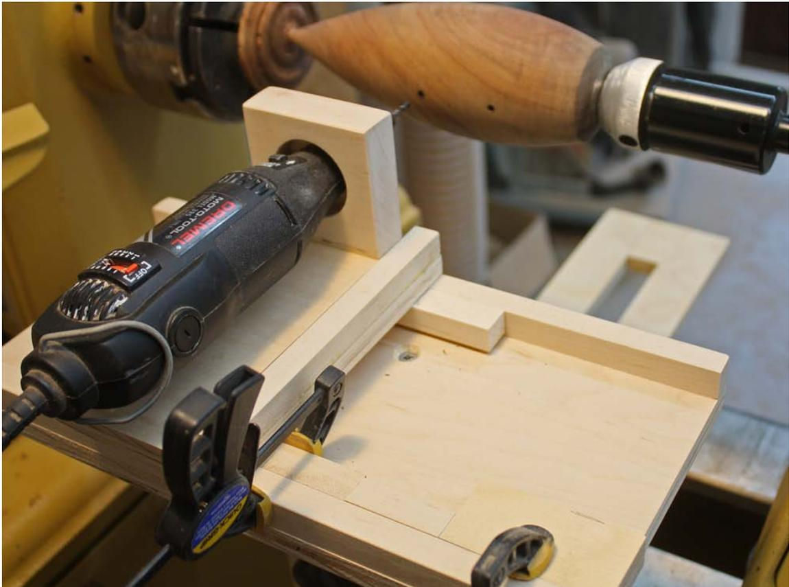
In this instance 2 mounting holes are drilled on each side of the vessel. Using the indexing feature on the lathe, the vessel has been locked in place. One hole is drilled and the spacer is inserted to drill the other hole. The vessel will then be rotated 180 degrees and the process repeated.
